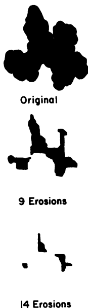
Figure 5: Pixel stripping routines called erosion routines can “dissolve” the image of a profile into probable constituent parts. (Reproduced with permission from ref. 2. Copyright 1990 VCH Publishers.)
